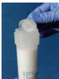
2 - Remove the PPHD Insert
