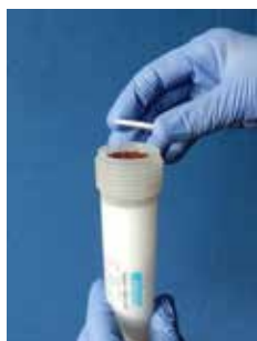
4 - Put the extra frit on top of your sample
